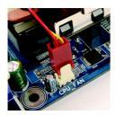
Please connect the heat sink power connector to the CPU\_FAN connector located on the motherboard so that the heat sink can properly function to prevent CPU overheating.
